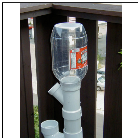
Solar stills can provide fresh water in an emergency, or water for on-board plants and hydroponics systems.
