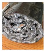
Roll forming using bubble pack and carbon or graphene separation allows assembly to become a battery or super-capacitor.
